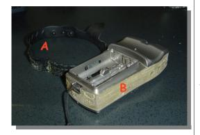
**FIRST REMOVE THE BATTERIES!** Carefully remove the "Rubber band" (A) from around the case. The adhesive is gummy and messy so take care. I used a knife blade to carefully lift and remove the band ... taking care not to cut the band during the process. There will then be a residue of the adhesive covering a clear vinyl tape around the joint (B).
