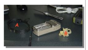
Next carefully remove the gummy adhesive and the clear vinyl tape from around the seam. This will leave you with a pile of "gunk" (B). Care should be used not to get this mess everywhere ... this would be a good time to use something to clean your hands to keep from smearing this everywhere.
